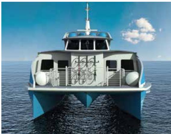
*Above: Engineering model of the completed Water-Go-Round ferry, which will be the first fuel-cell vessel in the Western Hemisphere and the first commercial fuel-cell ferry in the world. The Water-Go-Round is a 70-foot aluminum catamaran that will have a top speed of 22 knots.*
