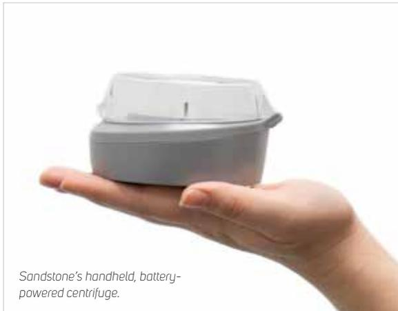
*Sandstone's handheld, battery-powered centrifuge.*
