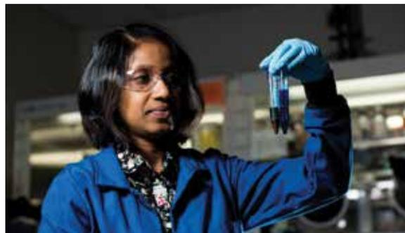
Above: A PNNL scientist examines electrolyte samples after exposure to 50°C temperature. The conventional vanadium electrolyte (vial on the left) has destabilized, forming solid precipitates that cause battery failure. PNNL's bi-additive electrolyte (vial on the right) remains stable from -5 to 50°C (an 80% improvement).
