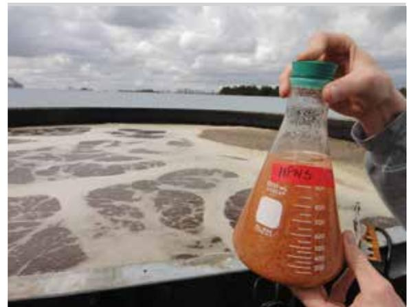
**Above:** Rapid start-up of a nitrification tank in a swine farm in North Carolina using 1L HPNS bacterial composition in 230 m3 liquid manure.
