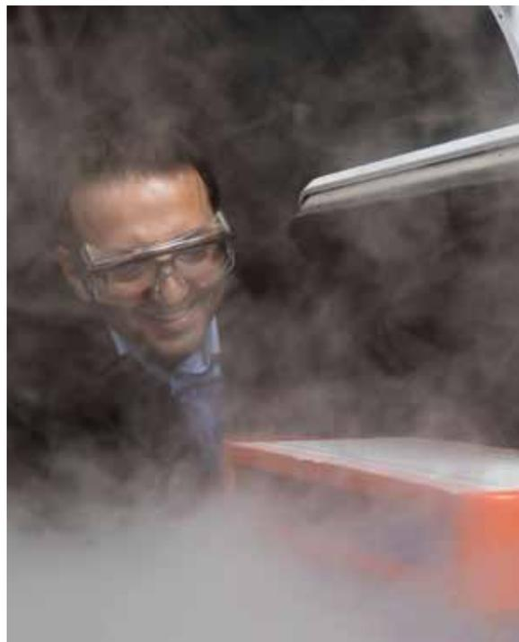
*Above: Dr. Ayyoub Momen, inventor and entrepreneur, demonstrates the press-type flatbed ultrasonic dryer developed at ORNL. The unit's piezoelectric transducers vibrate at high frequency, converting the water into tiny droplets that leave the fabric as a cool mist that resembles steam but without the energy required to change the water from liquid to vapor. (Credit: Oak Ridge National Laboratory)*
