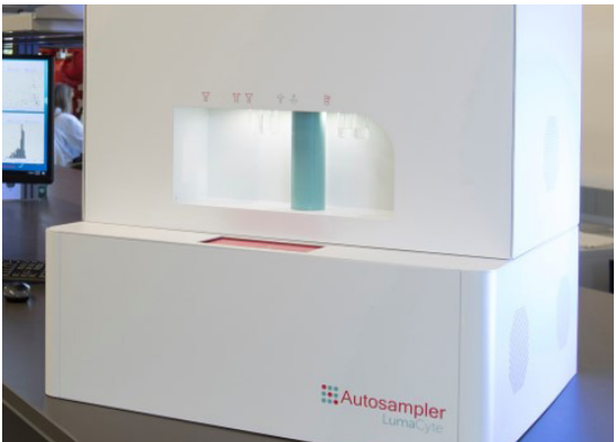
LumaCyte’s Radiance™, shown with an optional auto-sampler, utilizes Laser Force Cytology (LFC) based upon NRL’s LASI technology.
