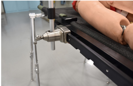
Drawing from the example of the common Picatinny rail system used on all military firearms, Drs. Hiles and Sirkin envisioned the SHRAIL as a universal platform on which medical personnel could quickly and consistently mount whatever equipment they needed to treat a patient in austere emergency situations.
